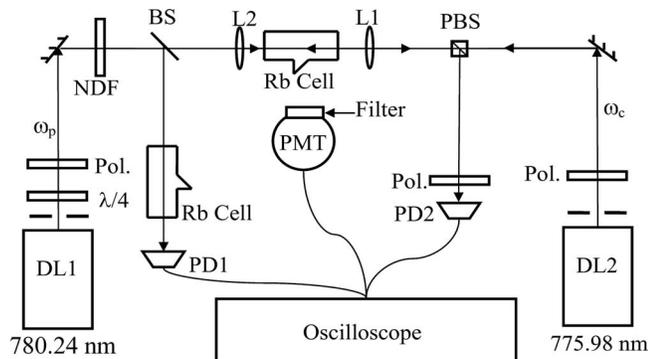
Fig. 5. Apparatus for the ladder-type EIT experiment. Components include grating-feedback diode lasers (DL), quarter-wave plates ( $\lambda/4$ ), linear polarizers (Pol), neutral density filter (NDF), beamsplitter (BS), polarizing beam splitter (PBS), lenses (L), rubidium cells, and photodetectors (PD). The fluorescence detection equipment (optional) includes a 420 nm interference filter and photomultiplier tube (PMT).
